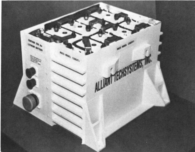
Fig. 1. A high power lithium thionyl chloride battery for space applications.
